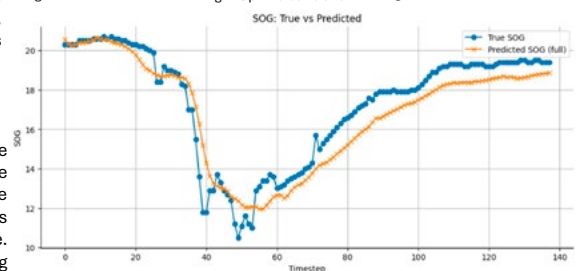
Fig 4: True speed over ground (SOG) vs. predicted speed over ground for an upwind maneuver.
